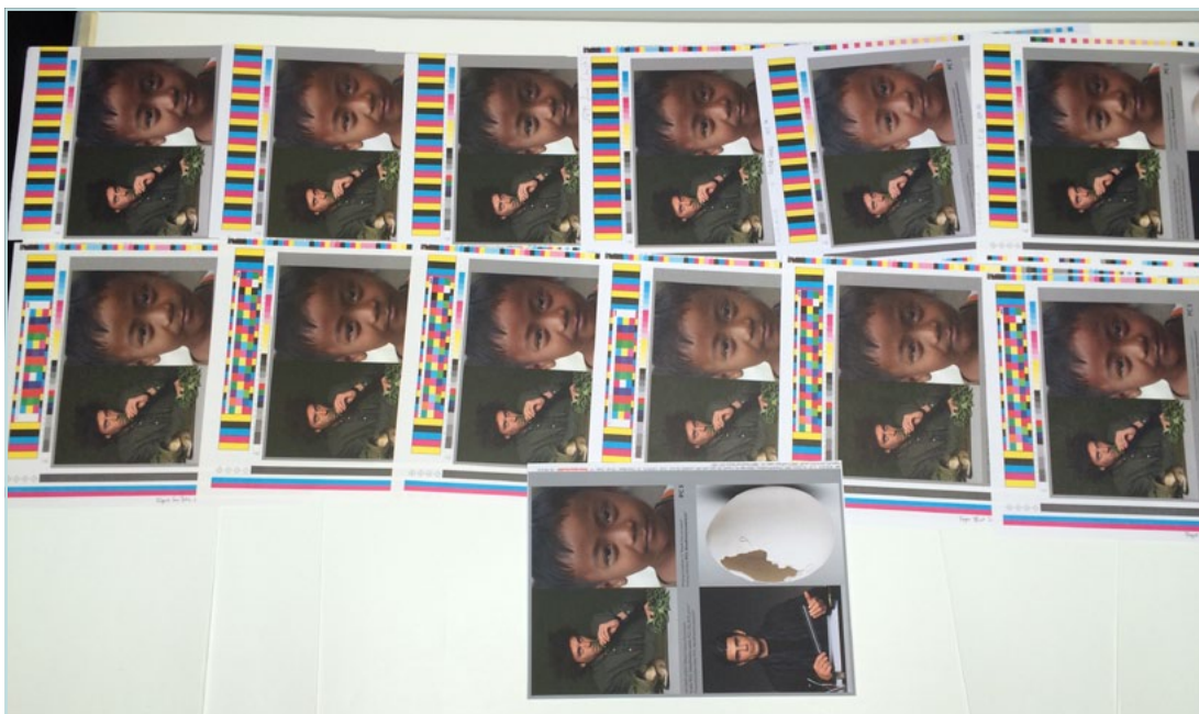
◀ Fig. 4: Comparison of different print samples for two motives. On the bottom center is the FOGRA52 proof. The visual differences are very prominent in the skin tone of the boy, even if it has to be noted that this motive reacts to even the smallest process fluctuations already.
